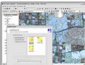
Use LoadBuilder to allocate demands using customer meters, service polygons, and more.
